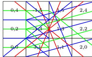
Figure 7: Arrangement after folding and interleaving shown divided into cabinets/racks. Colour key: North, East, South West
