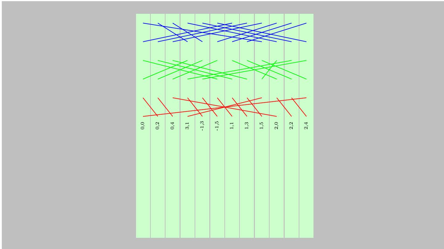
Figure 8: Allocation of SpiNNaker boards to cabinets and racks and the wires between them. Colour key: North, East, South West
