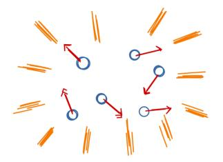
Generate particles with random positions in the target function space traveling at random velocities.
