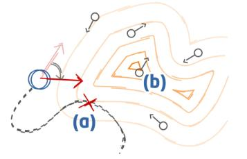
Update each particle's velocity using the best position that particle has been in (a) and the best particle in the swarm (b) with random weights.
