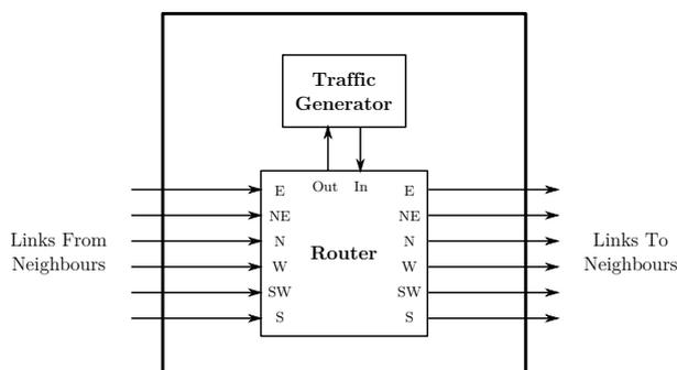
Figure 4: A node in the simulator representing one SpiNNaker chip. The traffic generator models all 18 ARM cores.
