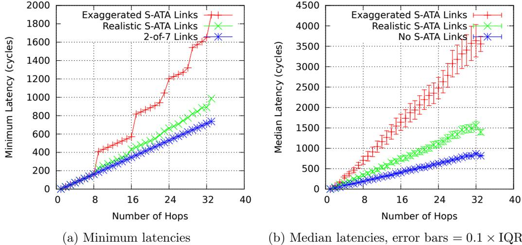
Figure 9: Latency for packets travelling along paths of varying lengths when boards are connected using different types of link.
