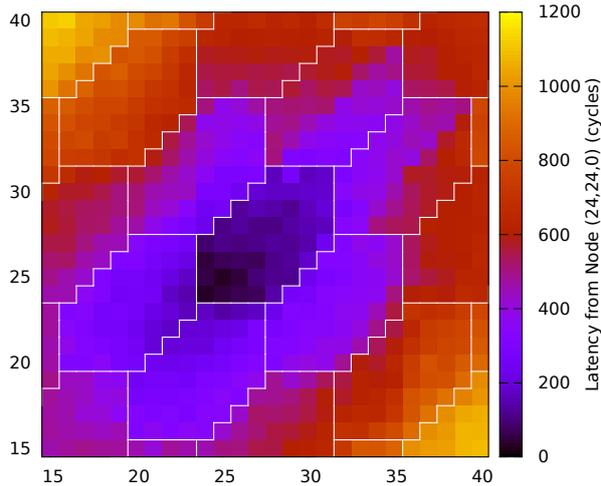
Figure 12: Heat-map of packet latencies from central node (24,24,0) on an unloaded system. Pixels are chips, white outlines are drawn along board outlines. The effects of border-unawareness in routing are visible as a step-change in latency along the diagonals of the upper-right boards. The S-ATA latency in this system has been exaggerated to aid visibility but is still present when realistic S-ATA latencies are used.
