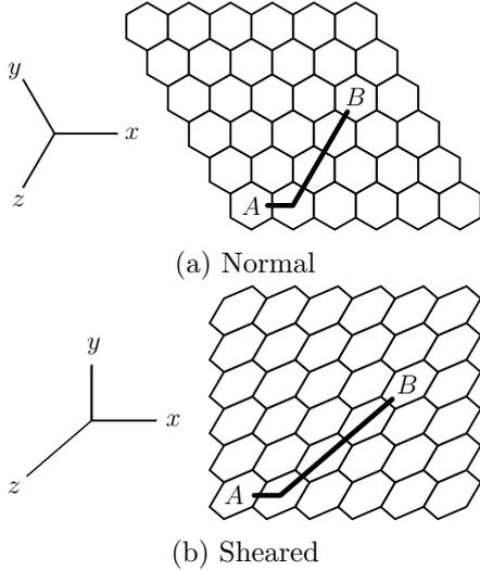
Figure 6: An example of a shortest-path between A and B on a hexagonal mesh. Shown both normally and sheared to yield the familiar 2D-mesh style layout. Note that the Z axis elongated which can make interpreting distances unintuitive in this projection.
