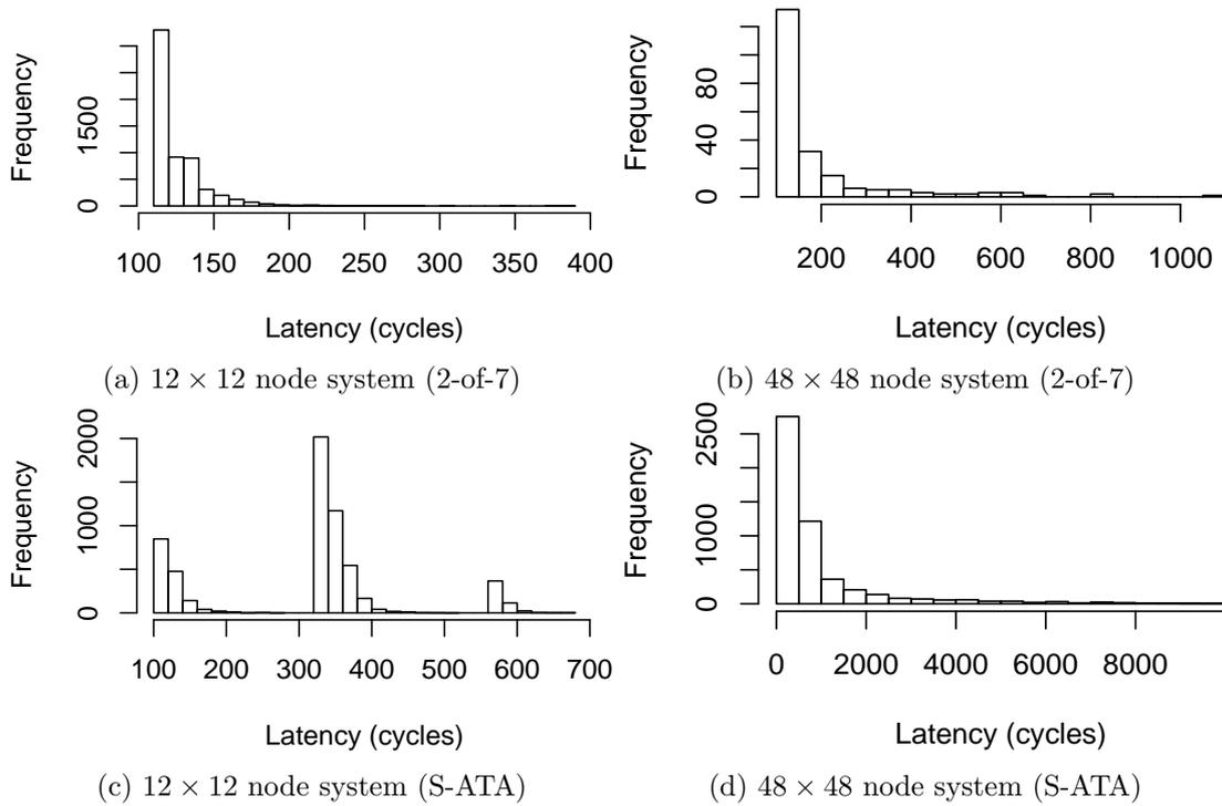
Figure 10: Histograms of packet latencies for 6-hop paths on different system sizes. (a) and (a) were simulated on a system using only 2-of-7 links. (c) and (d) were simulated on a system with boards connected via S-ATA links with exaggerated latencies.
