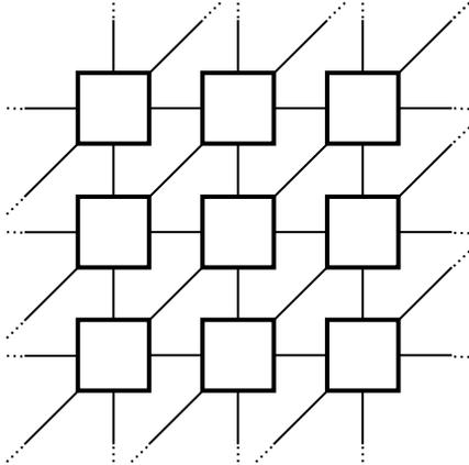
Figure 1: Chips in the SpiNNaker system are connected to their north, north-east, east, south, south-west and west neighbours. Connections on the extreme edges of the system are connected together forming a torus (not shown here).
