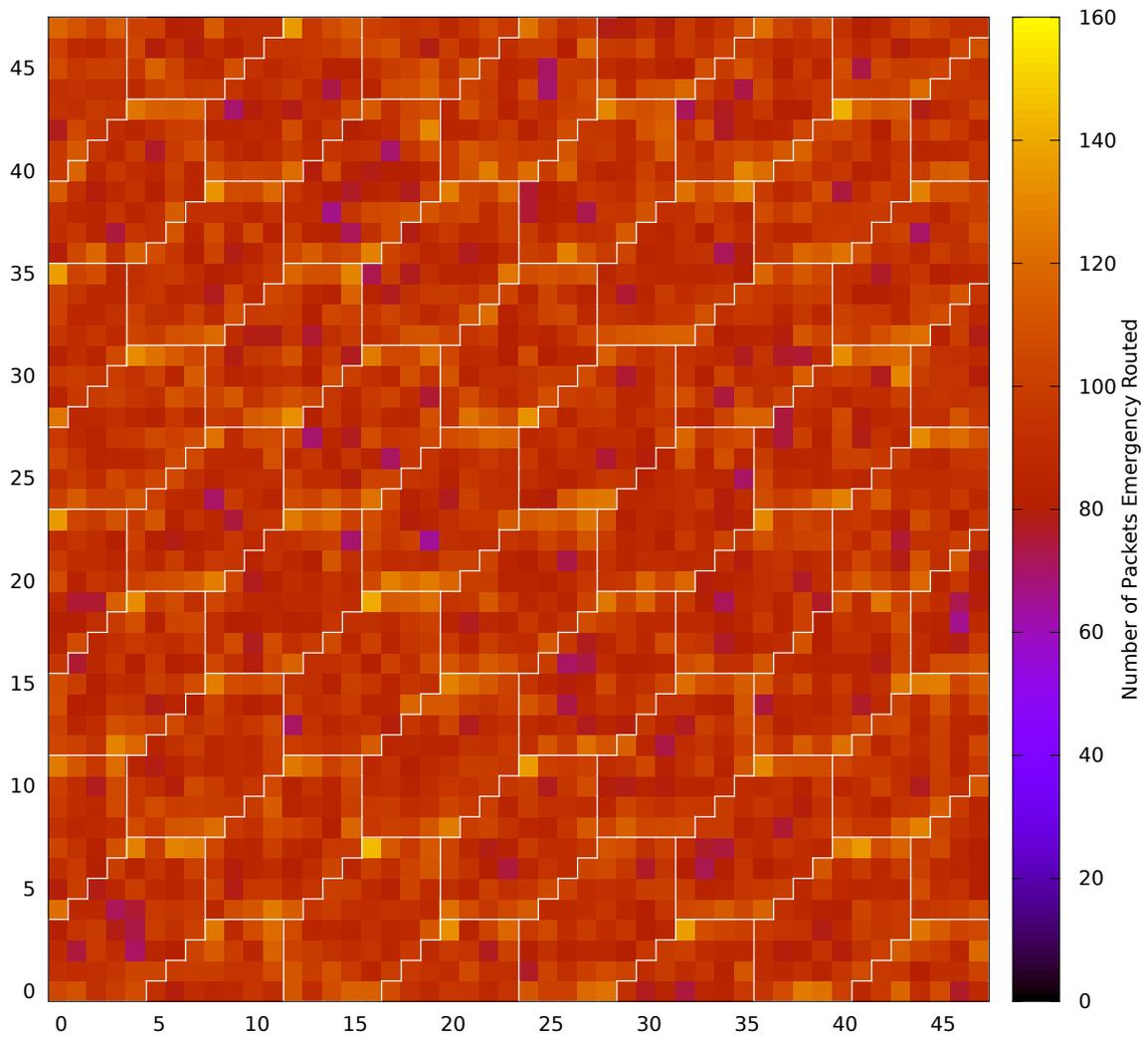
Figure 13: Heat-map showing the emergency-routing usage in a normally loaded system after 20,000 cycles. Hotter areas are visible along horizontal board edges.
