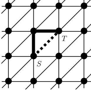
Figure 5: When sending a packet from node  $S$  to  $T$ , an emergency route (thick line) is used if intended link (dashed) is blocked for too long.
