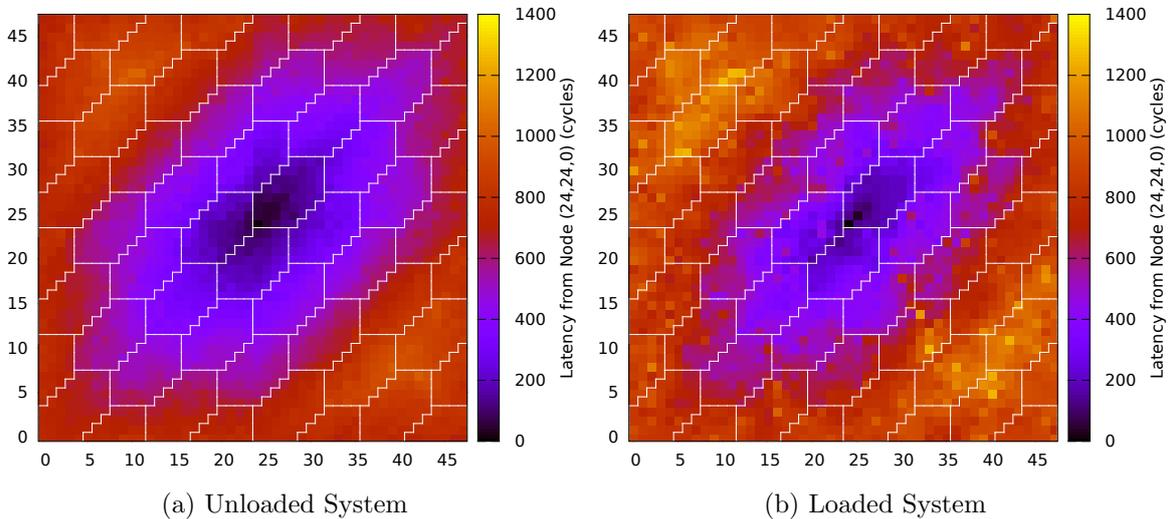
Figure 11: Heat-maps showing the packet latency from the central node (24,24,0) to the rest of the system. Each pixel represents a node in the system, the boundaries of boards are outlined in white. Note: A small number of randomly distributed nodes did not receive a packet from (24,24,0) during simulation due to packets not arriving within the simulation's execution. For clarity, the colour of these nodes has been interpolated.
